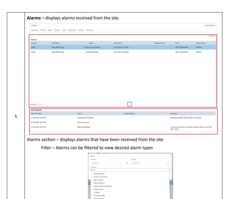
Alarm Details – select (highlight) an alarm and the details of that alarm will display at the bottom of the page
